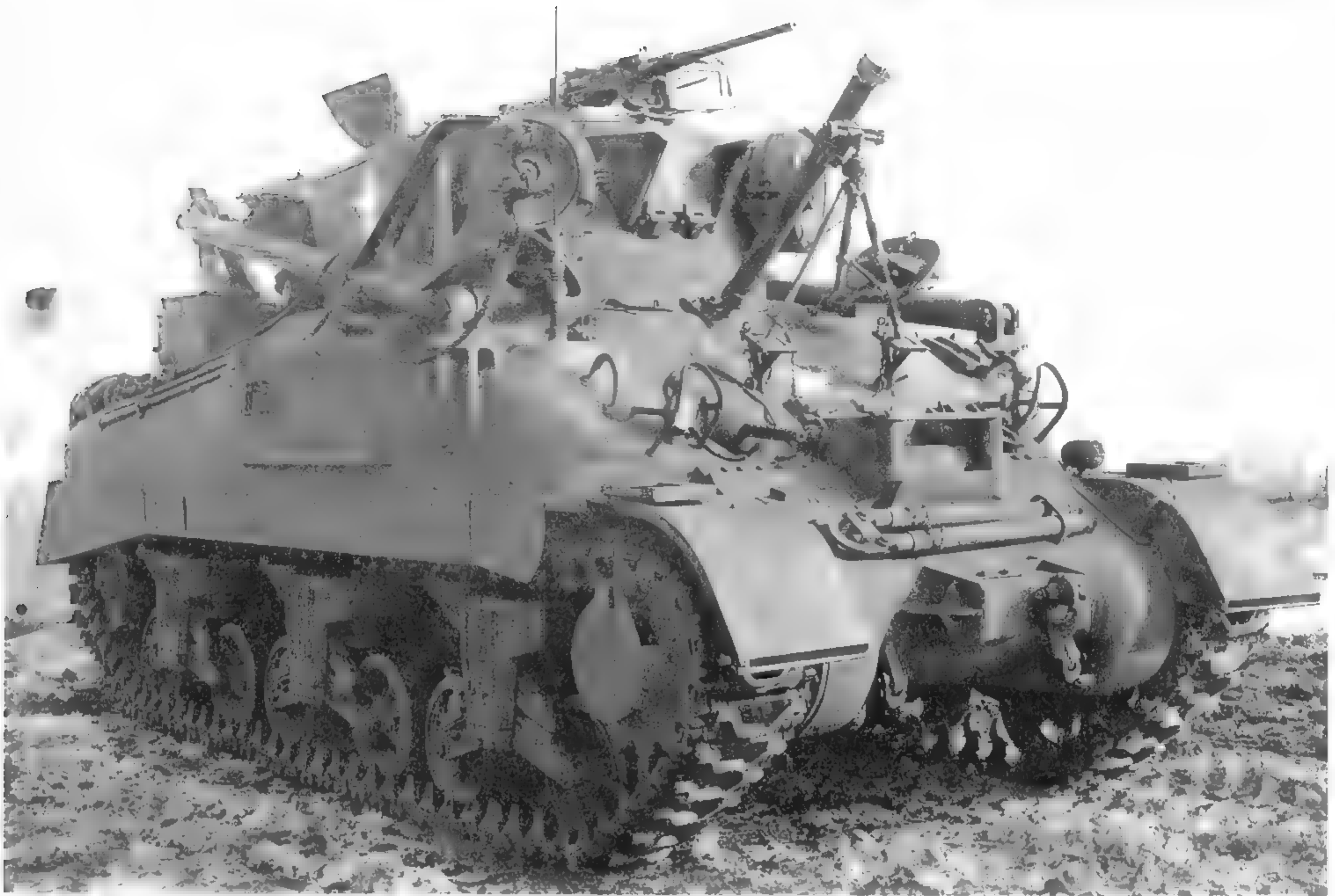
The M32B1 had the flexible .50-caliber machine gun on top, a ball-mounted .30-caliber machine gun, and an 81mm mortar on the glacis plate. The M32B1's cast hull M4A1 Sherman heritage is clearly evident. (U.S. Army photo)
